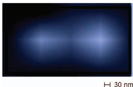
Figure 4. The polarization interferometric shape signal from two nano particles.
